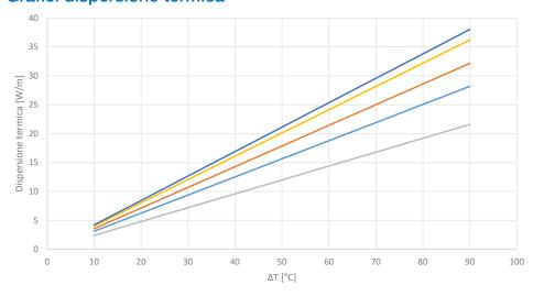
$\Delta T = \frac{\left(T_{v} + T_{r}\right)}{2} - T_{o}$
